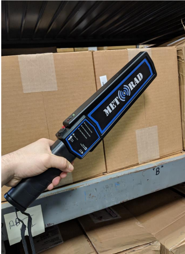
MetRad 1: Handheld Metal and Gamma Radiation Detector
